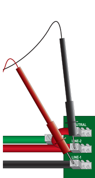
Line-2 and Line-1 240VAC (216VAC-264VAC)
