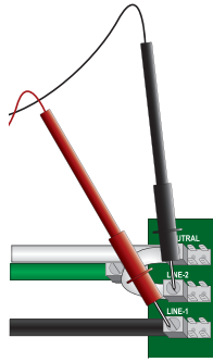
Line-2 and Line-1 120VAC (108VAC-132VAC)
